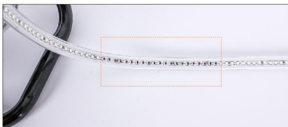
Puncturing the LED strip will damage the electrical circuit and cause LED failure
