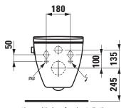
Connection with Laufen installation system LIS CW2
