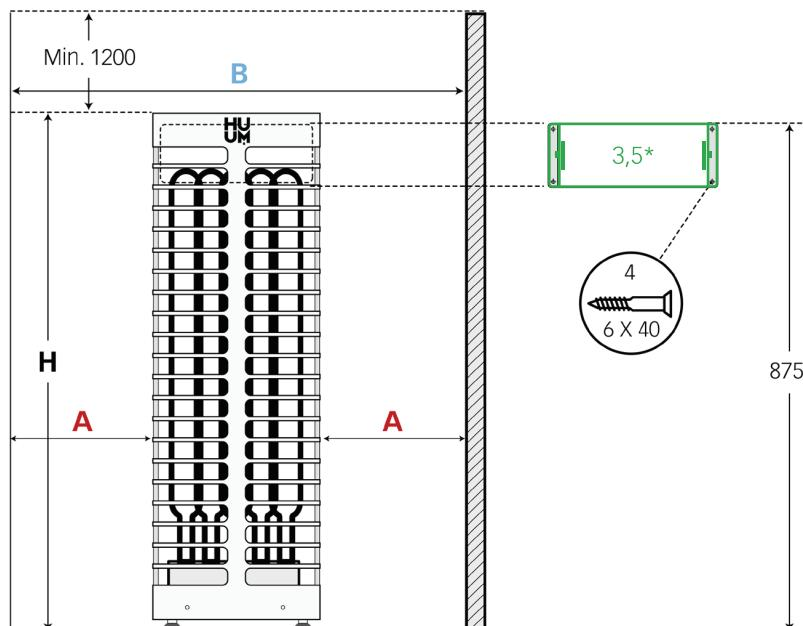
\* STEEL 3,5 is attached to the wall with a special bracket
