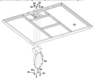
Install the backboard brace S, T on the back of backboard CC as shown.
