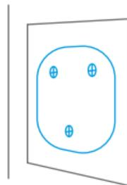
3. Drill the holes, insert the includes anchors and fix the mount to the wall as shown.
