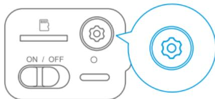
Open the cap at the bottom of the device and hold the **RESET BUTTON** for 5 seconds until you hear a beep. After resetting, all data will be deleted and the camera will reboot, allowing you to add it as new.
