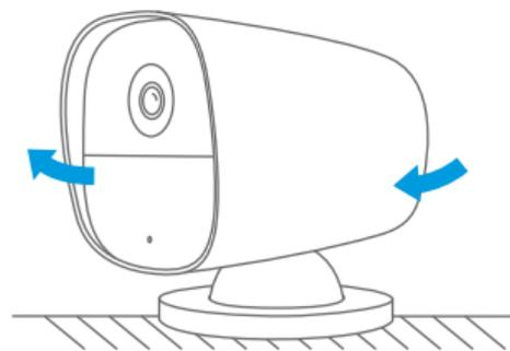
2. Rotate the camera to adjust the viewing angle.
