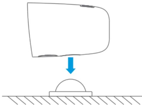
1. Place the magnetic ball mount on a table, shelf or any other flat surface and attach the camera on top of it, using its bottom base.
